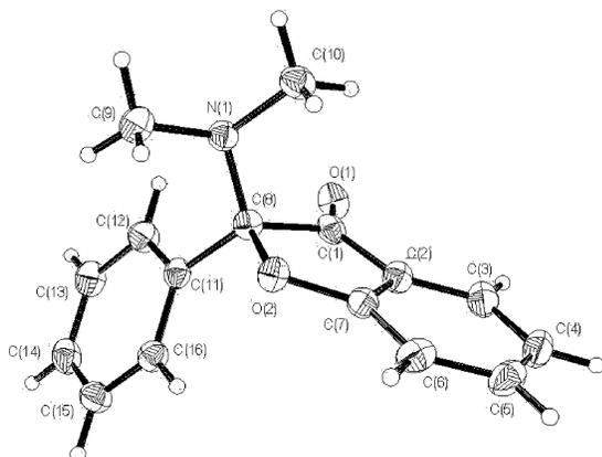
**Figure 3.** ORTEP representation (50% probability) of **3**. Selected bond lengths (Å) and angles (deg): C(1)–O(1) 1.2136(15), C(1)–C(8) 1.5612(17), C(8)–O(2) 1.4867(14), C(8)–N(1) 1.4312(16), C(8)–C(11) 1.5203(17); O(1)–C(1)–C(8) 123.66(11), C(1)–C(8)–O(2) 103.61(9), C(1)–C(8)–N(1) 111.65(10), C(1)–C(8)–C(11) 107.97(10), O(2)–C(8)–N(1) 111.10(9), O(2)–C(8)–C(11) 108.78(9).
